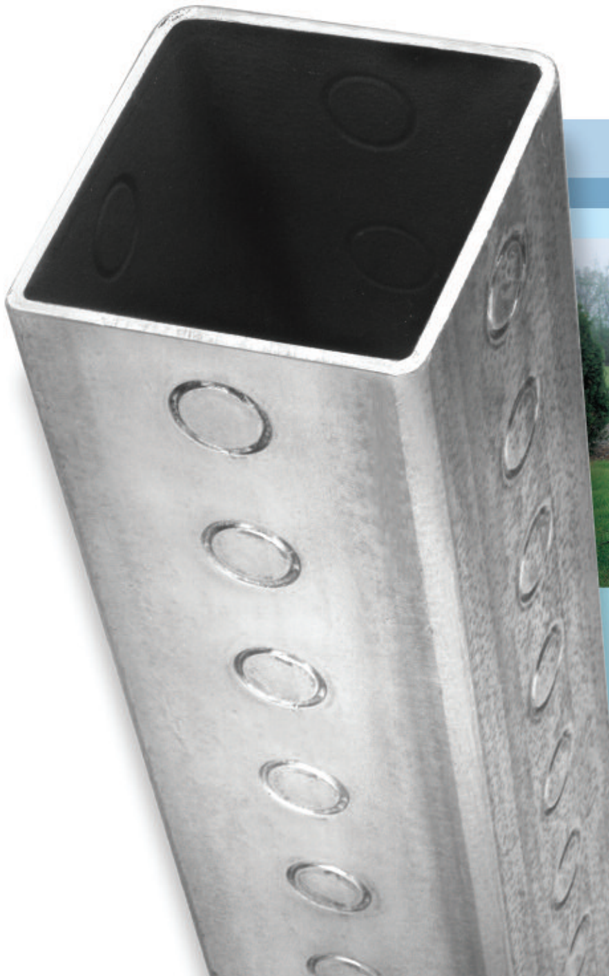
A minimum 30" piece of 12 gauge Telespar square steel tubing one size larger than the intended signpost is driven into the ground until 1-2 inches is left above the surface.
